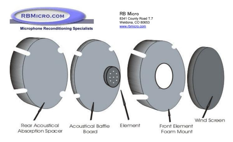
Instructions to install the MC-320 replacement element kit for an Astatic D104 head.
