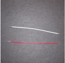
(d) When pre-tinning the wire that you are planning to use for the  $+ \log$  on the element, load end that was stripped 1/8" up with extra solder. This will allow it to be attached quickly when applying heat to soldering lug.
